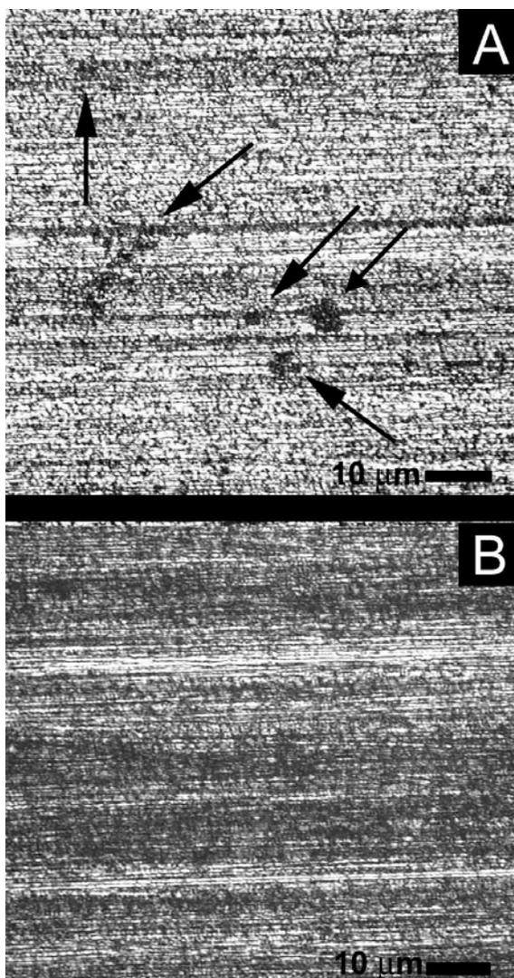
**Figure 8.** Polarized light image of 2 μm thick Ni pastes at the same magnification. A) Poor dispersion showing Ni agglomerates (arrows). B) Good dispersion showing no agglomeration. (Terpinol-cellulose type paste.)
