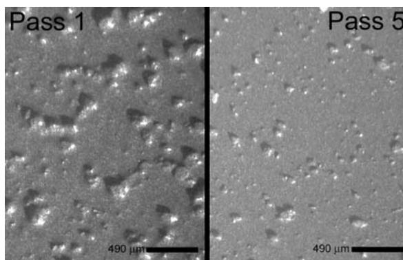
**Figure 7.** Low angle light (LAL) image of poorly dispersed Ni powder after 1st and 5th pass on a three roll mill.
