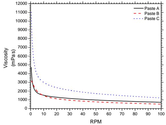
**Figure 4.** Viscosity responses of Ni electrode pastes after three roll milling (from Figure 3).
