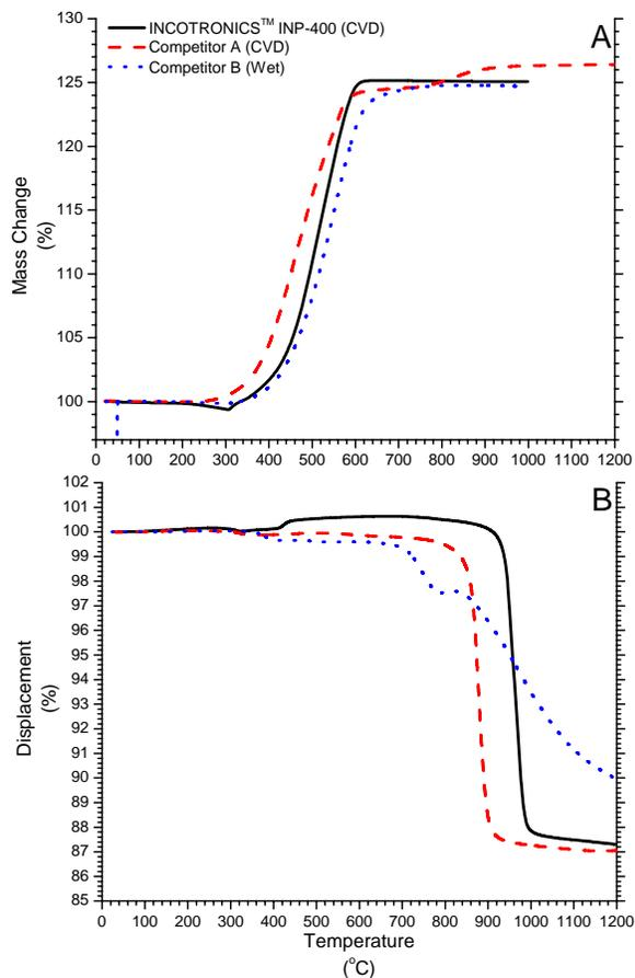
**Figure 2.** Comparison of thermal results of three different Ni electrode powders. A) TGA with scan rate of  $10^{\circ}\text{C}\cdot\text{min}^{-1}$  in air and B) TMA in  $1\% \text{H}_2\text{-N}_2$  at scan rate of  $10^{\circ}\text{C}\cdot\text{min}^{-1}$ .
