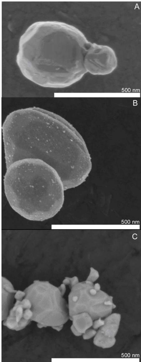
**Figure 1.** FESEM image of A) Incotronics™ Ni powder, B) CVD competitor powder, and C) wet process competitor powder. Magnification: 110,000X.
