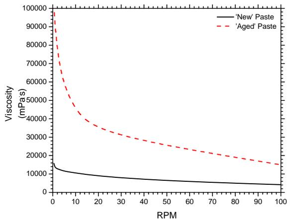
**Figure 6.** Viscosity responses of Ni electrode Paste B (Figure 5) showing dramatic aging effect.
