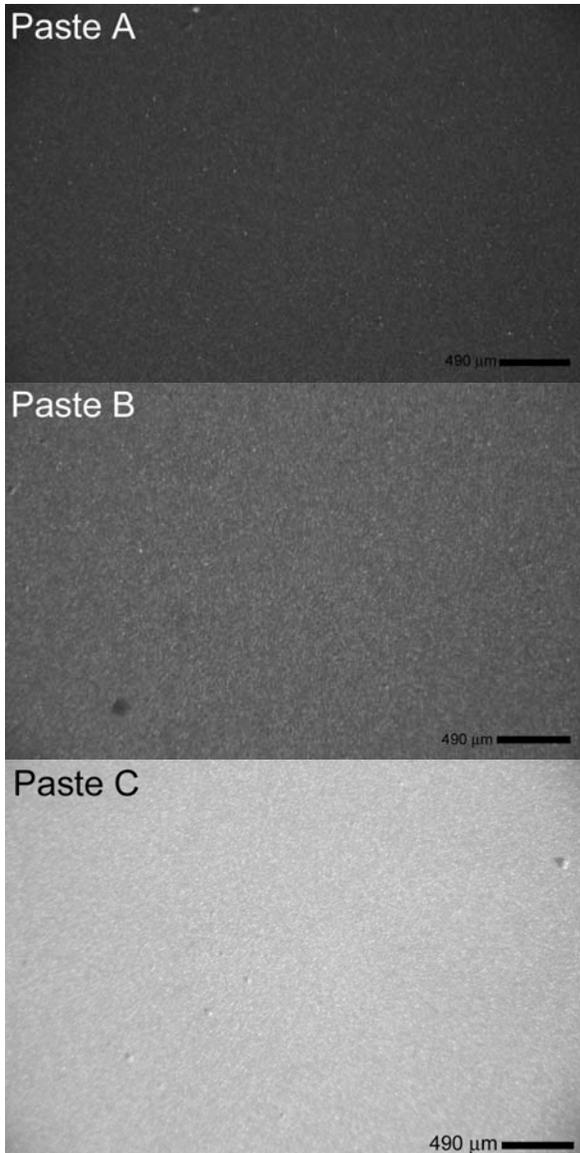
**Figure 3.** Low angle light (LAL) images of Ni electrode paste (from same Ni powder) in three different vehicle systems.
