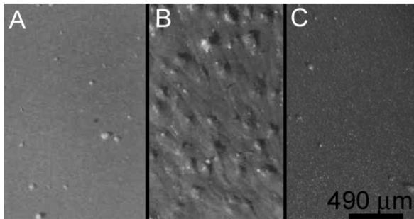
**Figure 5.** Low angle light (LAL) image of a Ni powder in three different vehicle systems. Paste A shows moderate behavior, Paste B shows very poor behavior, and Paste C shows good behavior.
