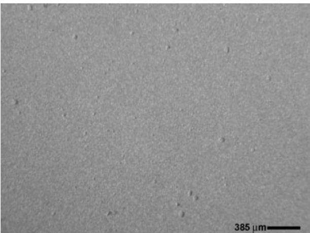
Figure 11. Typical LAL of Metalor CP0504. As seen from the previous figures (Figure 9 – 11), the high silver CP0504 produces a good smooth electrode when printed with a simple cellulose vehicle.
