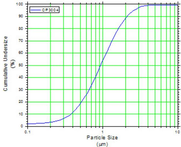
Figure 4. Typical PSD image of Metalor CP3004 (70%Ag30%Pd)
