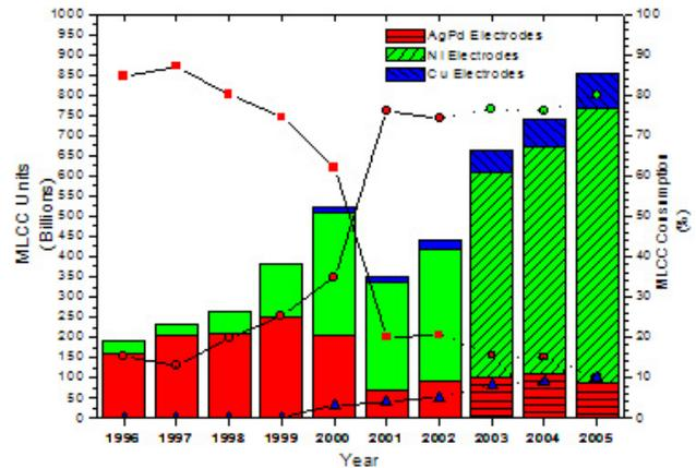
Figure 1. Past MLCC consumption trends and future projection for devices made with AgPd, Ni, and Cu electrodes.
