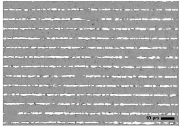
Figure 6. Cross section of 0402 (X7R) MLCC for a 47 nF device with a 10 V operating voltage made with Metalor CP3004 electrode powder.
