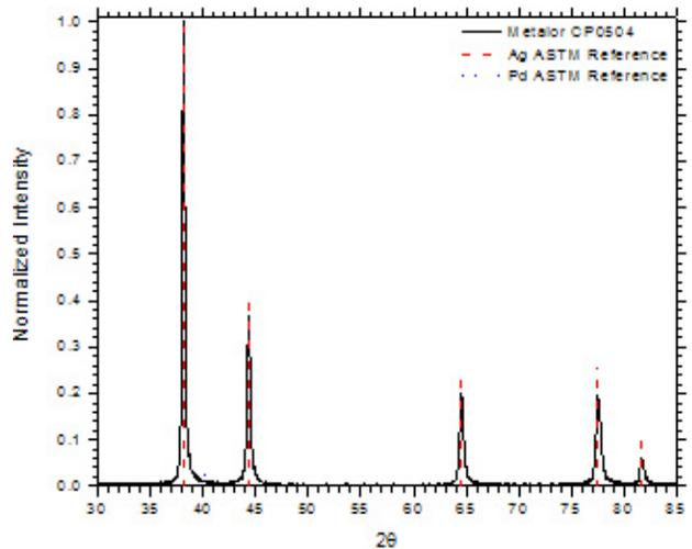
Figure 12. XRD spectrum of Metalor CP0504 (95%Ag05%Pd) electrode powder.
