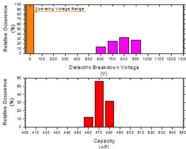
Figure 14. Electrical results for a 0804 (X7R) MLCC part made with Metalor CP0504 electrode powder
