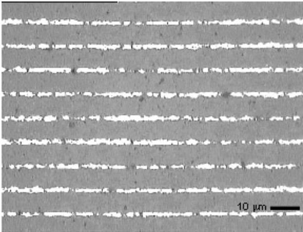
Figure 13. Cross section of 0804 (X7R) MLCC.
