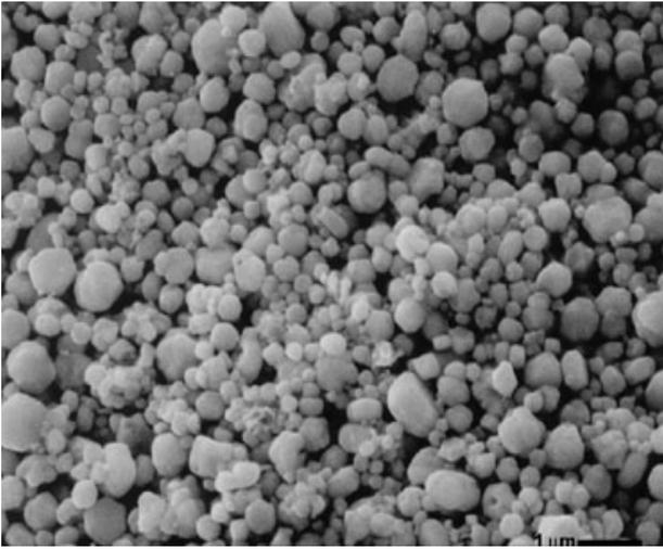
Figure 9. Typical SEM image of Metalor CP0504 (95%Ag05%Pd).
