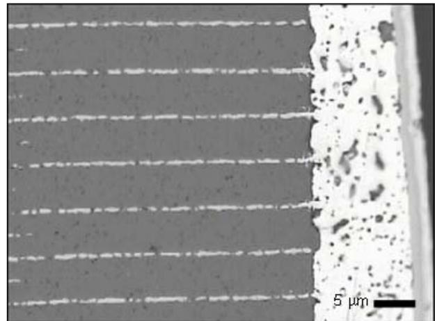
Figure 7. Cross section of 0402 (X7R) MLCC showing good connection between electrode and termination.
