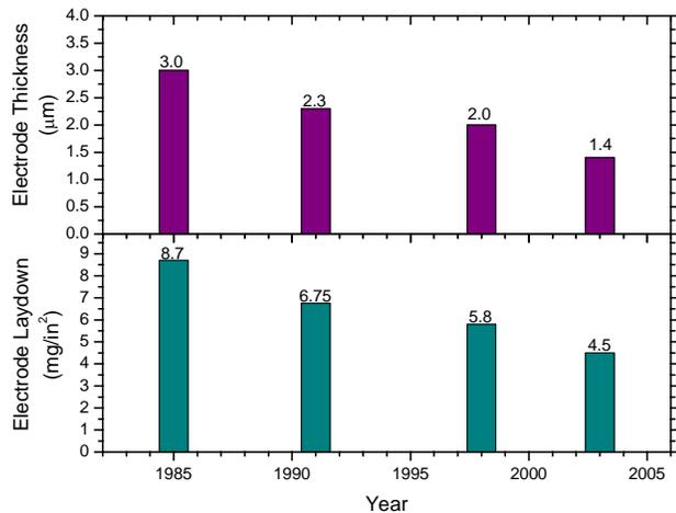
Figure 2. Historic MLCC trends for AgPd electrode laydown and thickness.
