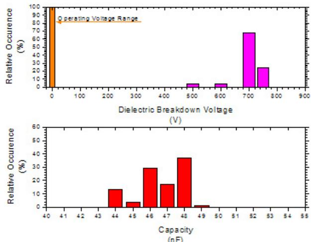
Figure 8. Electrical results for an 0402 (X7R) MLCC part made with Metalor CP3004 electrode powder.
