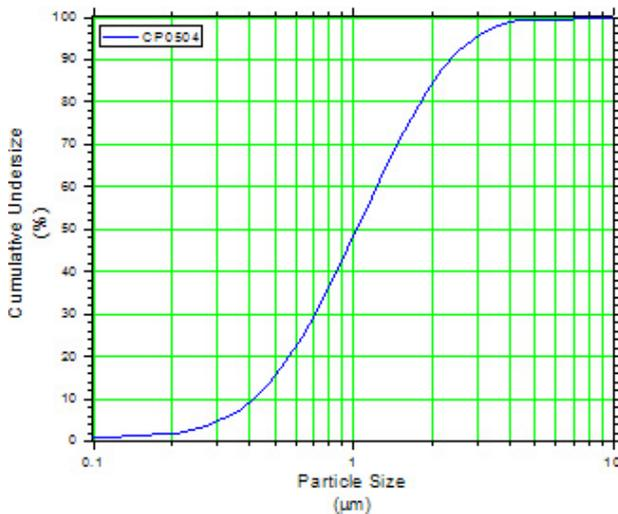
Figure 10. Typical PSD of Metalor CP0504.
