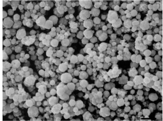
Figure 3. Typical SEM image of Metalor CP3004 (70%Ag30%Pd).
